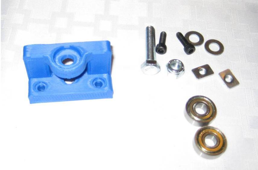
**Step 29:** Reinstall the stock Taz idler hardware, with the bolt head at the bottom of the idler block, followed by a washer, 2 608zz bearings, another washer, and then the Nut on the outside of the assembly as shown in the picture below.
