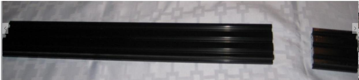
Measure your 500mm x 60mm x 20mm Openbuilds rail to ensure it is in fact actually 500mm long. If so, remove 64mm using a metal blade hacksaw and a miter box. The openbuilds X axis design allows for approximately +/- 2mm error on this cut.
