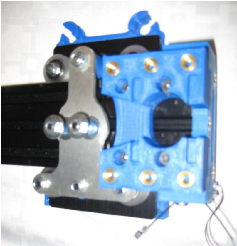
**Step 42:** Check for clearance of the X carriage on both sides, and alignment with the endstop.
