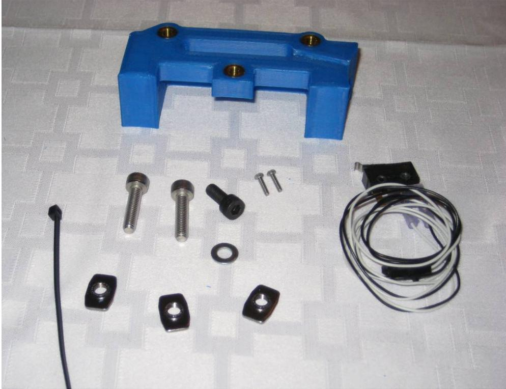
**Step 37:** Install the X minimum Endstop using the M2 bolts.
