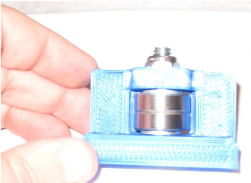
**Step 30:** Insert the M5 bolts through the assembly, and pre install the T-nuts. Set this assembly aside for now.
