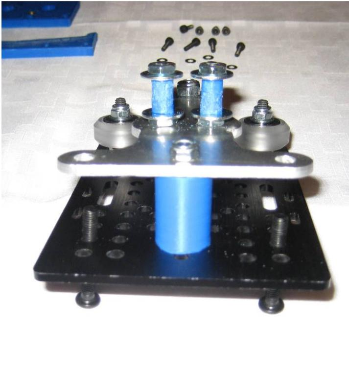
**Step 19:** Slip one of the 6mm non eccentric spacers over each bolt
