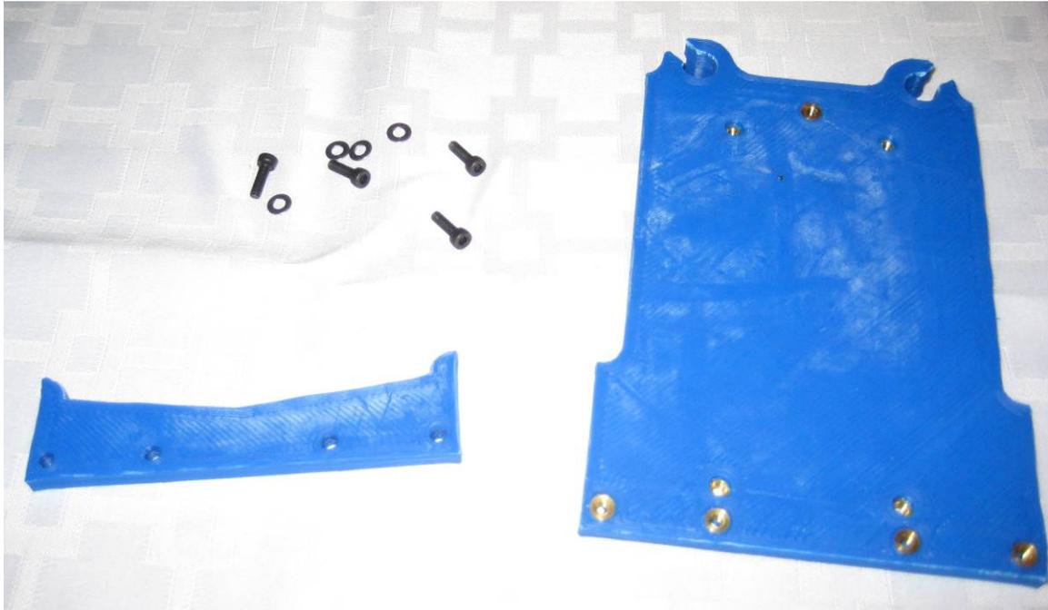
**Step 23:** Install the carriage guide to the adaptor plate, ensure that the notch slopes down towards the plate so that it mirrors the stock configuration
