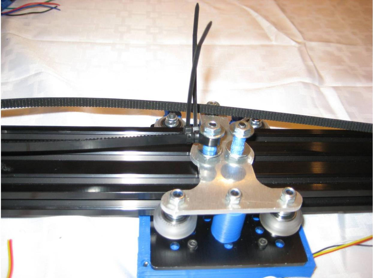
**Step 48:** Attach the motor mount lid to the main block, with the belt around the motor pulley. Adjust the motor position as needed using the M3 screws until you get a smooth belt path that isn't blocked.
