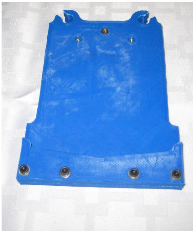
**Step 24:** Flip the adaptor plate over, locate the 4 8mm M3 screws, and position the X carriage gantry plate and back plate assembly so that the bolt heads line up with the recessed circles
